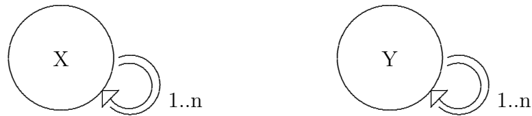
Figure 9.12: The two networks for predicting x and y zone position. 1..n indicates that there are n temporal links, each going one step further into the future than the previous.
